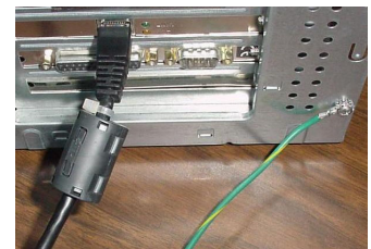
This partial view of the host PC shows the Ethernet cable with a ferrite collar. The PC's connection to the ground-line is also visible.
